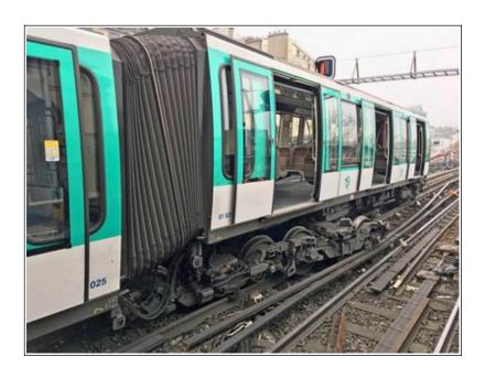
On Friday 2 December 2016 at 12:01 pm at the Barbes-Rochechouart station on line 2 of the Paris metro, the fourth and fifth cars of a train travelling in the direction of the Porte Dauphine derailed when entering the station. Damage to infrastructure and rolling stock was significant. No passengers were injured in the accident, nor during evacuation of the train.
