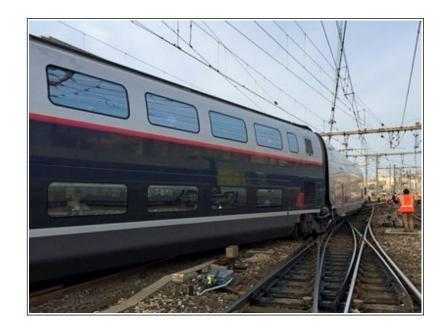
Friday 24 August 2018, just before 6:00 pm, the TGV 6145 coming from Paris arrived at the Marseilles Saint-Charles station, its terminus. The TGV was made up of two elementary trainsets coupled in a multiple unit. As the train was travelling 28 km/h and the front already reached the platform, the rear train derailed with the last seven cars and the last power unit.
