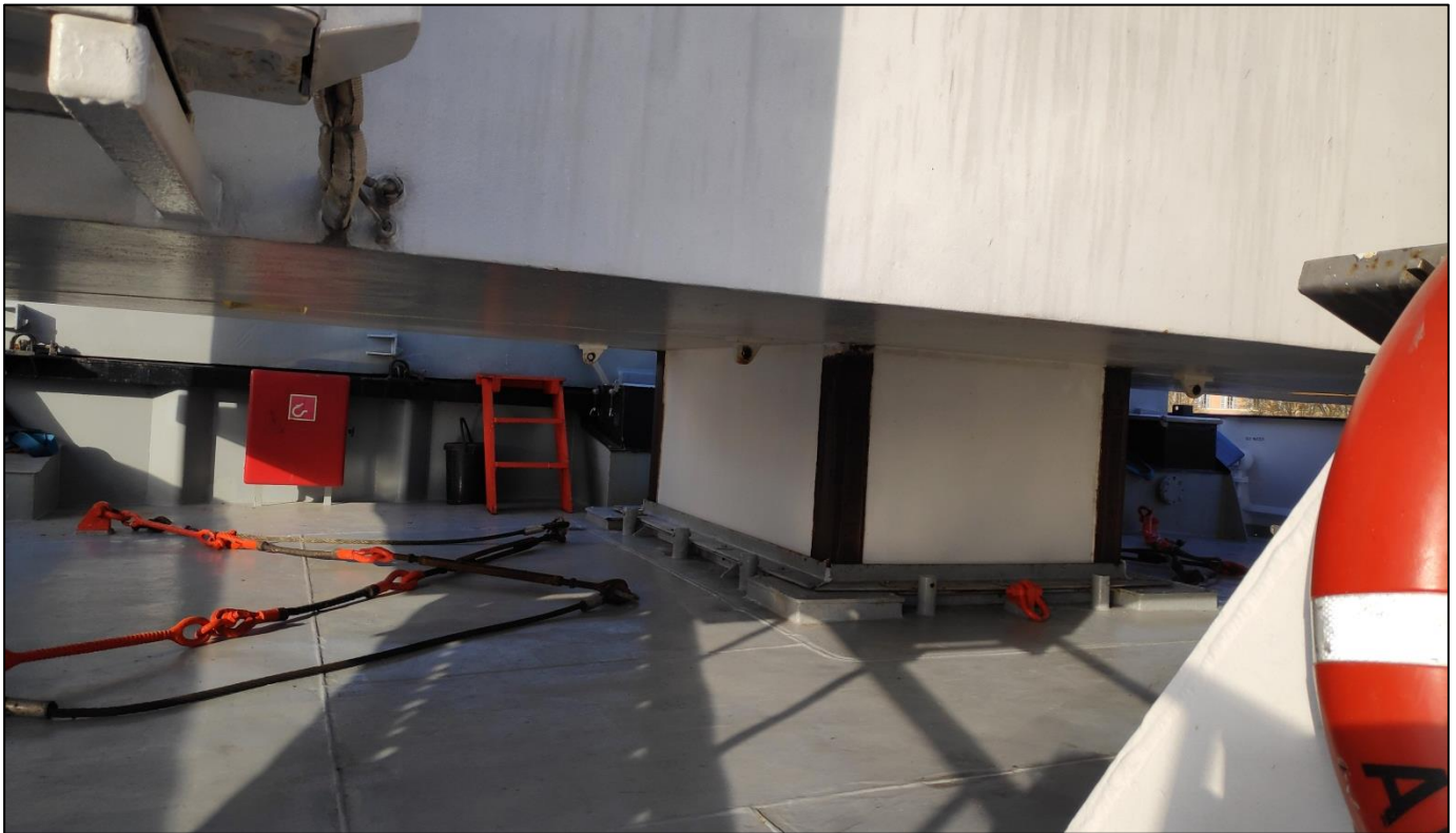
Telescopic base of the wheelhouse
