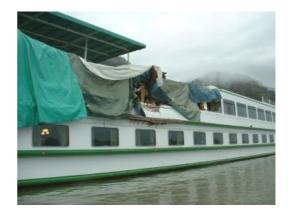
At 02.28 am on 28 March 2006, the CAMARGUE passenger boat, with 138 passengers and 25 crew members aboard, struck a pier of the railway viaduct at La Voulte-sur-Rhône when passing underneath the bridge. The impact caused significant damage to the superstructures of the boat. Nine passengers were slightly wounded. The bridge sustained no notable damage and the accident had no impact on navigation.
